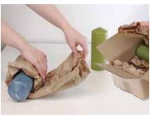
The PadPak LC is the fastest paper cushioning solution on the market. The high output allows a maximum box throughput. The converter forms single layer paper into pads which can be used to protect products during shipment. The individual fanfolded packs of paper, with gluing strip, ensure the converter is easy to load and runs at high speed. The paper pad can be used for cushioning, fixating or wrapping.
