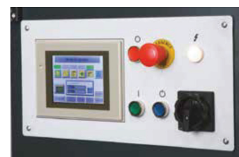
F-344 : Touch screen control panel for machine functions management
