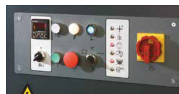
F-144 : Control panel with optic indicators of operation anomalies
