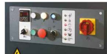
F-144 : Control panel with optic indicators of operation anomalies
