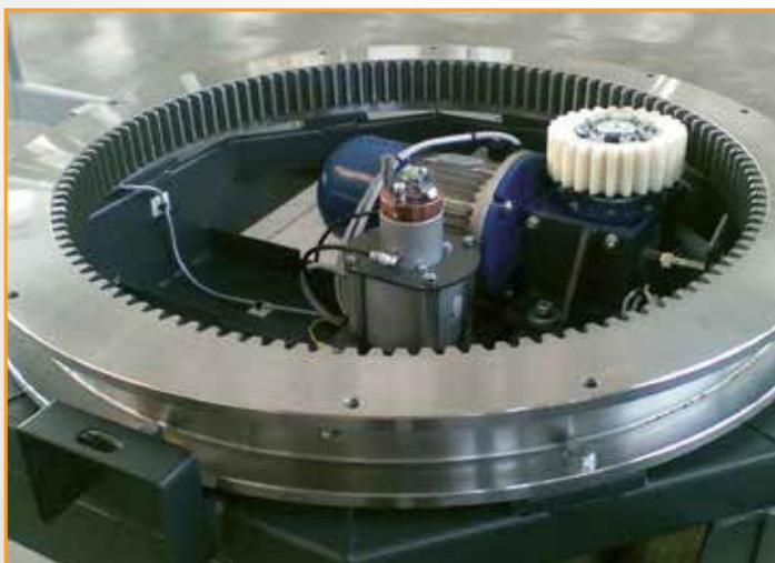
Strong "crown bearing" for turntable support and drives
